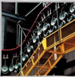
*mefro* wheels are iron phosphatized and powder coated in silver metallic. By this method the wheel's surface gains a very good protection against corrosion and an excellent finish. Top coating of all wheels in special colour shades is possible, provided appropriate quantities are involved. Out of environmental concerns we do not use any coating powders containing lead, cadmium or other heavy metals.
